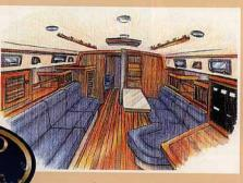
numerous opening ports, Dorade deck vents and hatches, and durable and easily maintained overhead and hull surfaces make this salon and the entire interior attractive, comfortable and practical.
